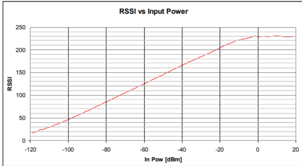
Figure 11: Input Power to RSSI Mapping for the RFM22B
