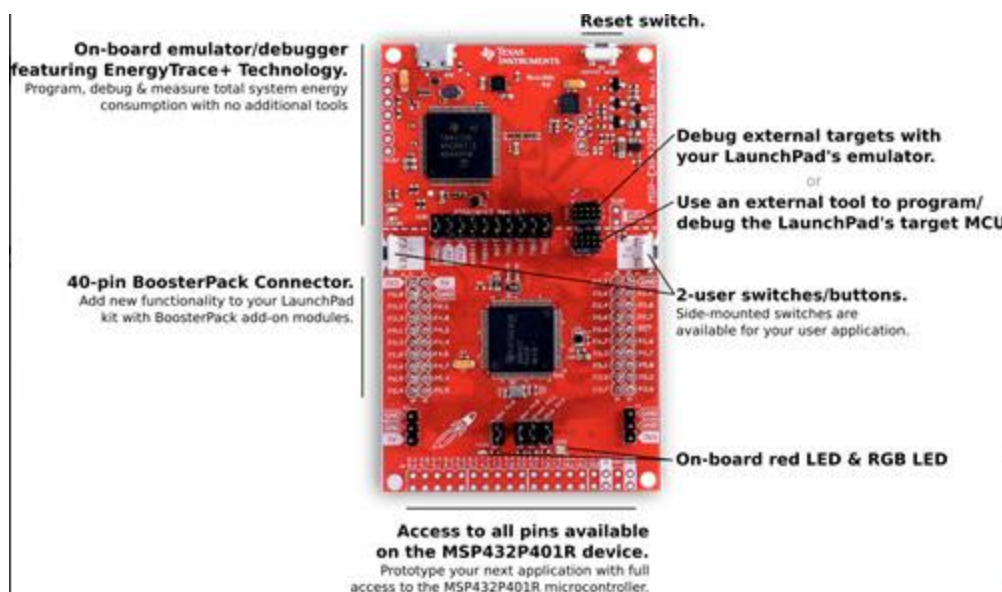
Figure 8: MSP432P401R Launchpad Development Board
